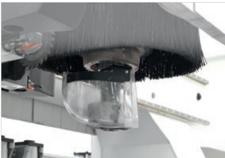
NC-controlled deflector (chip conveyor).
