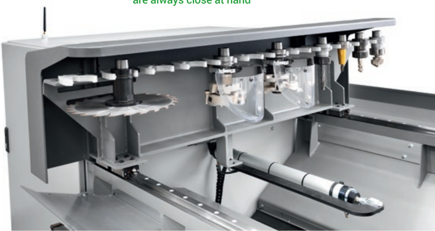
Rack tool magazine with 12 or 23 places, with integrated pick-up.
