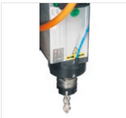
Fixed vertical motor dedicated to additional milling operations (slot, anti-splintering, etc.).
