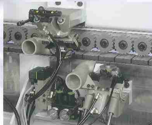
Profile scraper unit with quick release heads to facilitate tool changes.
