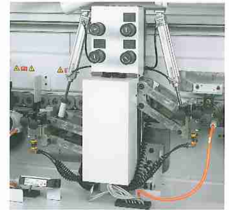
Profile trimmer with automatic adjustment for thin and thick edge materials.
