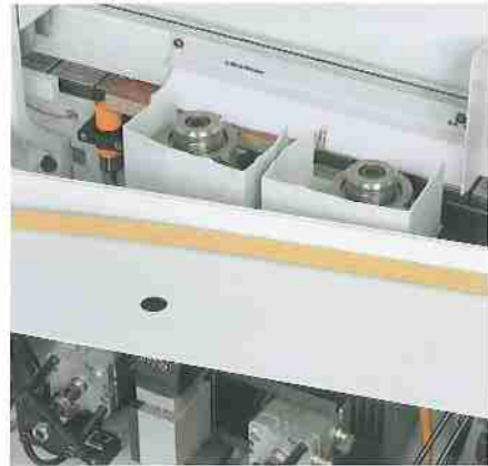
Joint trimming unit for finish trimming sawn or routed edges to achieve an optimum edge quality.
