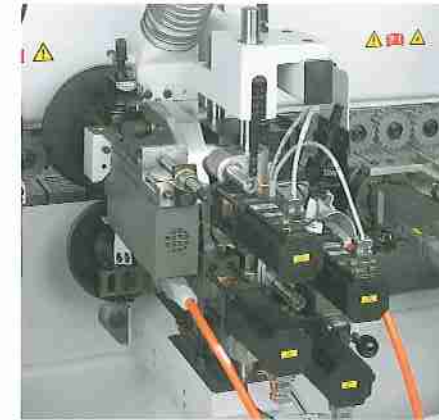
Flexibility for different edge material thicknesses and profiles by the use of NC servo motor positioning.
