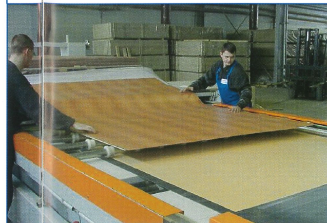
LAY-UP DEVICE Automatic board lay-up device and manual laying-up of the melamine paper
