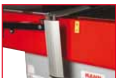
klappbare CPS Hobelwellenabdeckung CPS cutter block protection
