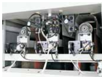
Schleifbandreinigung blower device to clear sanding belts
