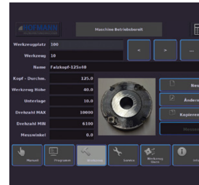
Tool mask display of tool data graphical representation of the tool
