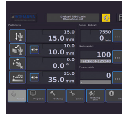
Spindle start variable speed preselection
