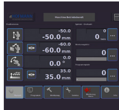
Tool change releasing the HSK interface via the touch control panel
