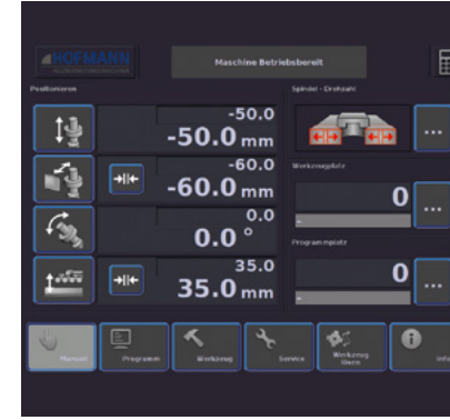
Guardian Monitoring of the stop jaw clamping in the CNC control
