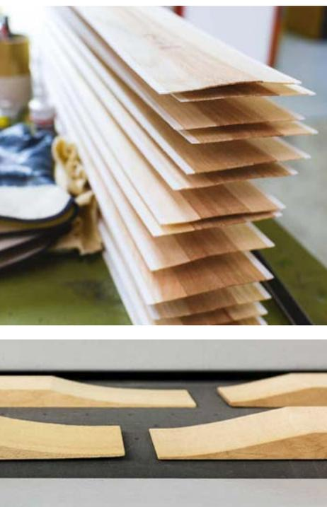
CNC sanding technology is another one of our innovations. It allows contouring with a repeat accuracy and speed that is unattainable with manual sanding or milling. The technology is well proven in instrument construction (for example guitar necks) and especially in production of skis and snowboards.
