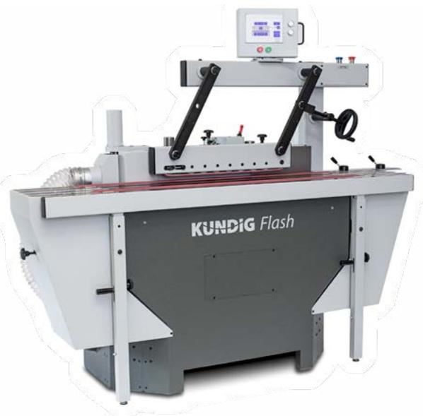
The **Flash** is specially designed for edge lacquer sanding. With the application-controlled, pneumatic sanding pad, belt blow-off jets and variable sanding belt speed, perfect lacquer sanding is achieved, even on high-gloss lacquered edges. The machine is operated via a touch screen which can be rotated by 270°.
