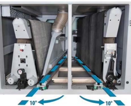
The engineers at KUNDIG have developed the „Vmax“ principle, which solves the challenges of sanding window frames. Two oblique units arranged in a V-shape ensure that the crossbar of the window frame never hits the sanding unit at a right angle. The technology has proven itself over the last 15 years at numerous window manufacturers. There are several advantages:
