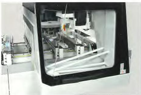
Working unit protection with transparent surfaces to enable the operator to safely view the entire working area.
