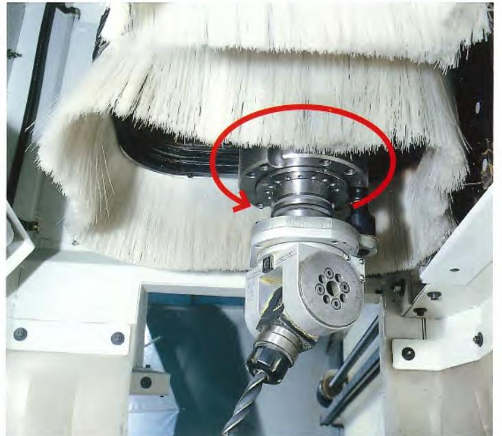
Interpolating Vector rotating axis (0-360°) enables the use of angular driven heads.
