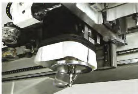
The new off-cut conveyor fitted on the electro-spindle tilts and turns according to the spindle's movements and conveys the machined off-cuts away from the working area and eliminates dust from the workplace environment.
