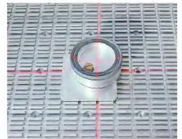
A series of threaded holes (120 mm pitch) provide perfect fixing for all hold-down devices.
