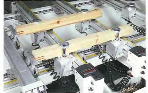
TVN SET is the ideal worktable for the automatic positioning of the bars for linear components such as doors, windows, staircases, beams, columns. Extremely simple and easy to use, this system combines the flexibility of clamping device manual positioning with automatic bar positioning handled by the CNC.
