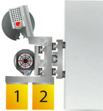
LOGICO machining head can be compounded with a wide range of functional modules in order to solve any machining need. With the tool changer on board, it drastically reduces the cycle times because the tool change occurs in masked time.
