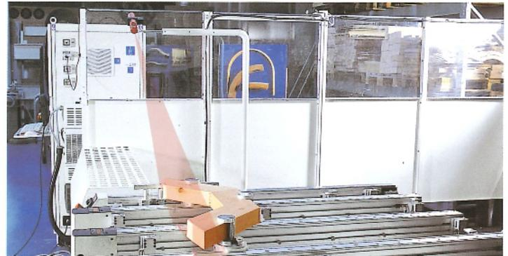
Guided by a laser light, the operator can easily position arched components.
