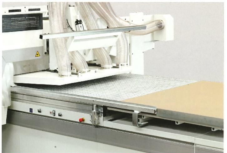
A special pusher, directly controlled by the program, ensures not only finished component outfeed but also a fast and automatic cleaning of the working area.
