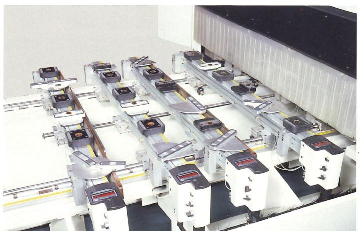
With the innovative pneumatic clamp quick release system on the bar, there is no need for tools and worktable re-configuration becomes extremely fast and easy.
