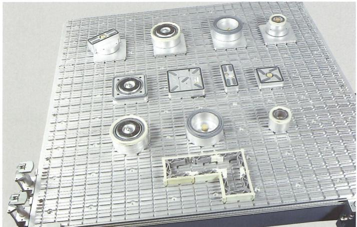
Utilising a laser positioning system, worktable set-up operations become easy and fast.
