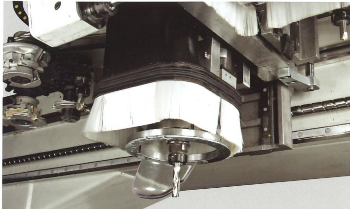
The new off-cut conveyor fitted on the electro-spindle tilts and turns according to the spindle's movements and conveys the machined off-cuts away from the working area and eliminates dust from the workplace environment.
