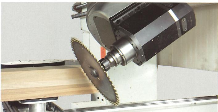
High power at low speeds. The Prisma unit is the perfect solution for saw blade cutting operations on solid wood.
