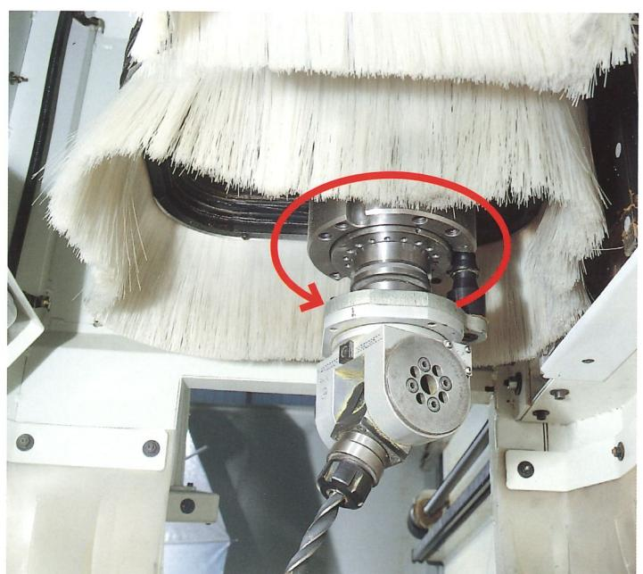
Interpolating Vector rotating axis (0-360°) enables the use of angular driven heads.
