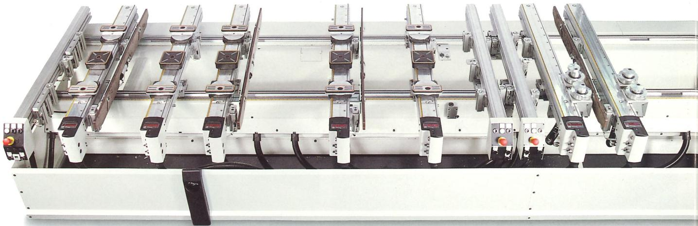
TVN worktable bars are the perfect solution for quick and safe component clamping: the bars can be fitted with quick release suction cups or pneumatic clamps for maximum ease of use.
