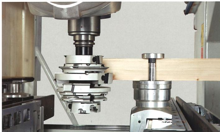
Machining with double profile tool reduces tool changes and increases productivity.
