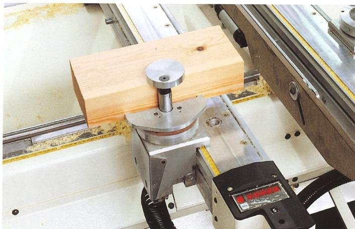
A special pneumatic clamp enables the machining of very short components.
