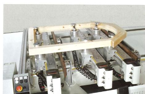
Quick release rotating clamps and double movement lifting units make it easy for assembled sash positioning and for trimming operations.
