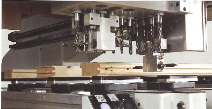
**F11, F18, F26:** a wide range of drilling units with independent drilling spindles specifically designed for drilling of solid wood.
