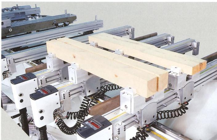
A solution for clamping each staircase component:
