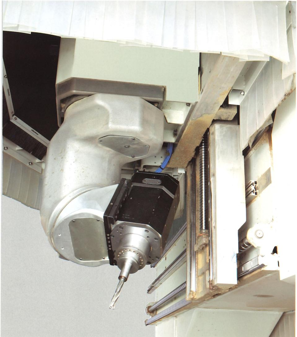
5 axis flexibility combined with 3 axis rigidity thanks to the **TTS** system.
