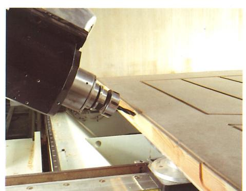
With the Prisma machining head, the same tool can be used horizontally, vertically or in any tilted angle. No need for auxiliary units, the reduction of tool changes and a faster production process.
