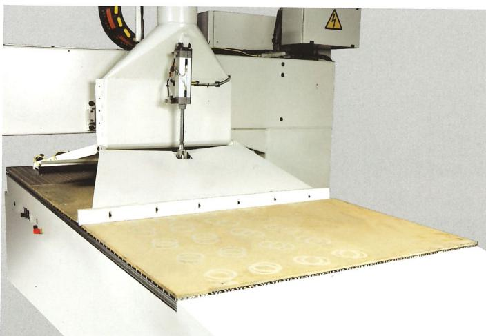
A special pusher, directly controlled by the program, ensures not only finished component outfeed but also a fast and automatic cleaning of the working area.
