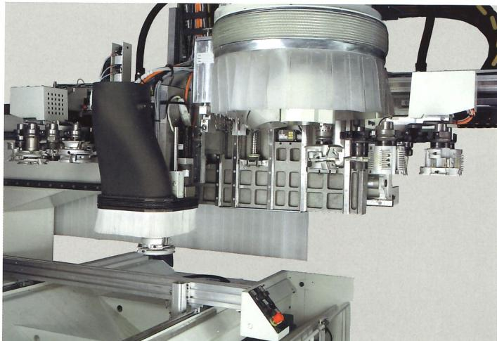
TECNO machining head considerably increases productivity enabling tool changing in masked time during other auxiliary unit machining cycles.
