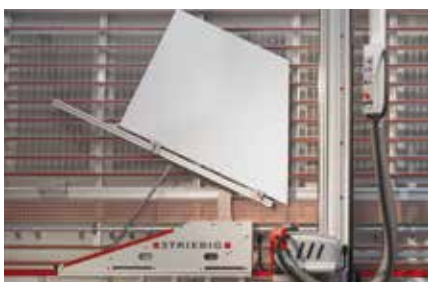
The angle cutting unit WSG maintains the set dimension accurately in all angle settings.
