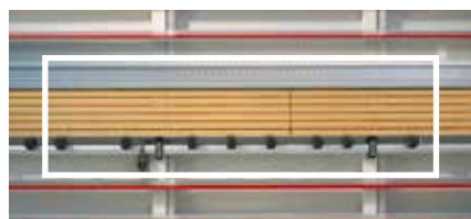
Continuous central and small parts support over the entire length for increased comfort while cutting small parts. Series: central support made of resistant aluminium grids. Option: high-end grids made of synthetic materials for especially demanding panel coatings.
