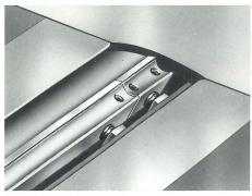
\*Tungsten Tipped Cutter Inserts Widens the scope of the machine, as difficult materials, eg. chipboard, formica etc., can be edged.
