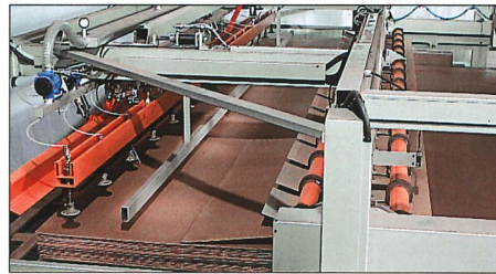
Rapid loading device with vacuum and nip rollers (optional).
