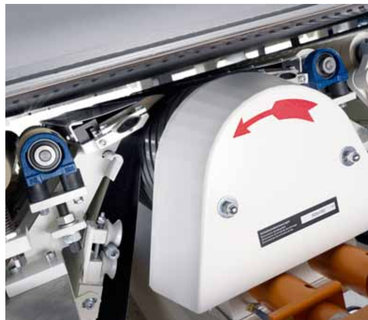
The contact roller unit of a LSM 8 sanding from below.
