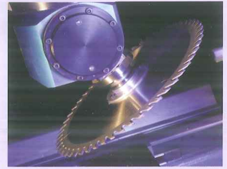
FLEX5 unit – automatic swivel angle setting, e.g. for shift cuts
