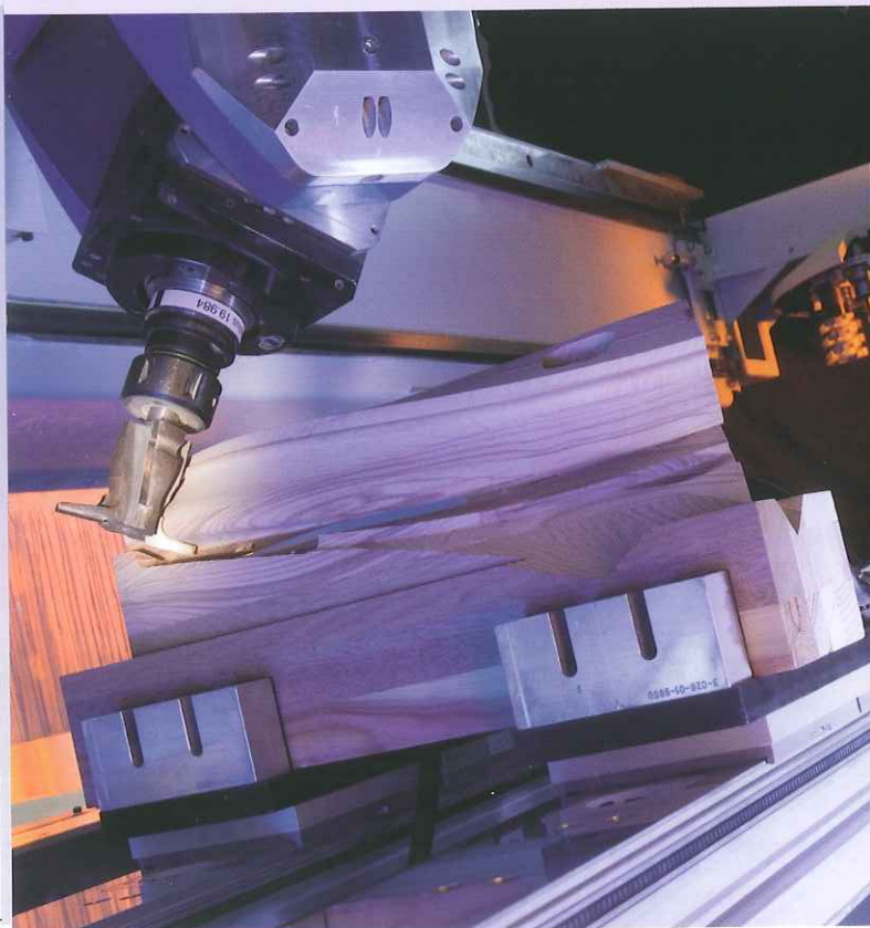
DRIVE5+: optionally 3, 4 or 5-axis trimming spindles with access to a maximum of 72 tools and units
