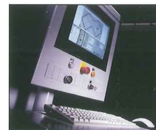
power control PC 85: with control panel for simple machine operation through features such as the graphic tool database and machine data acquisition (MDA)
