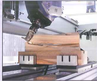
The high-rigidity extension arm design is configured for the DRIVE5+ five-axis trimming spindle with a maximum workpiece height of 300 mm – even with tool lengths of 230 mm (including HSK adapter)
