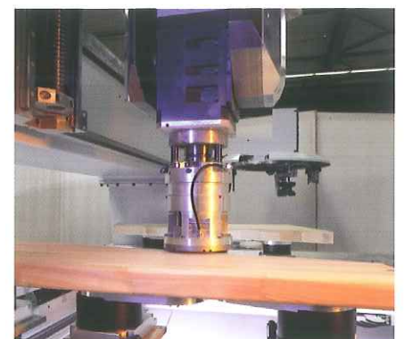
DRIVE5+ trimming spindle with vertically traced unit
