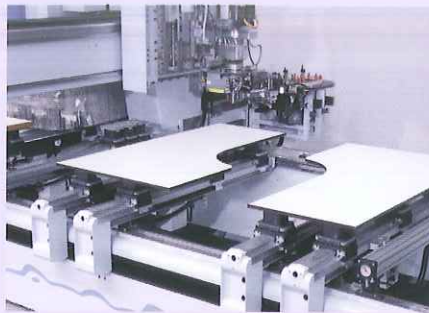
Lateral traversing of consoles after division of raw panels for edge banding
