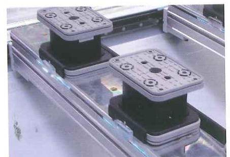
Console table for precise part fixture
