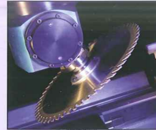
The ultimate in flexibility: the integrated FLEX5 interface permits retrofitting with the fifth axis at any time. A unique feature permitting the precise execution of shift cuts or drilling and trimming operations at "any" angle without the need for manual settings
