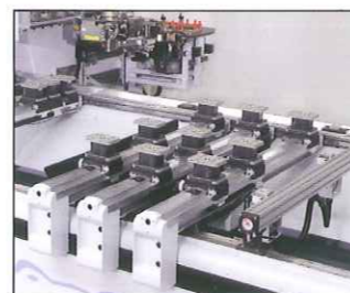
The automatic positioning table offers greater convenience, shorter set-up times and a range of additional functions such as moving workpieces apart after a dividing cut
