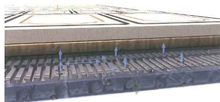
Air cushion function for simple handling of large-format workpieces
