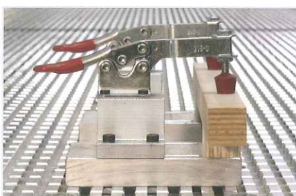
Grooved aluminium grid table guarantees precise fixture using mechanical clamping elements in any optional position
