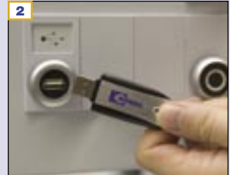
2 USB port For data input or data backup to an external memory. This allows the complete data set to be downloaded from the machine's control system and safely stored. The 1:1 data backup facility ensures that the system is immediately back up and running after an interruption.
