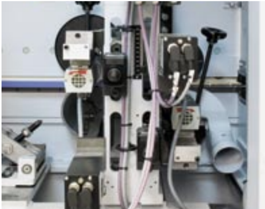
Trimming unit 0.4 kW (automatic instead of manual) for automatic program-based chamfer/radius adjustment
