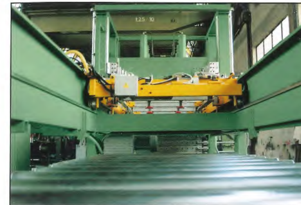
Detail of the vacuum unloading inside the KOMPAX press:
