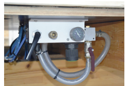
Includes pneumatics systems for the central air supply and controlling the C-PowerTec clamping beams
