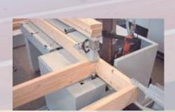
It all starts with the new WEM 100. In this model variation, the beams and studs are fed in manually. After that, the discharge gripper drives along for the distance given. The next stud is put in, then nailed, and the process starts again. This offers a convenient starting model for craftsmen's businesses or smaller industrial companies with a production capacity from 100 houses per year on. Optional supplementary modules such as a noggin station and studs in feed is possible.
