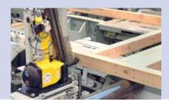
discharge gripper which moves exactly to the single stud positions. Another innovation are the freely definable nailing positions for different stud types such as L, U, T or multiple studs.
