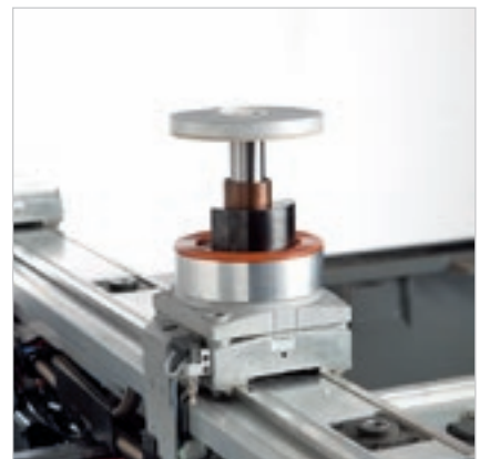
Hyperclamp for rigid and precise locking.
