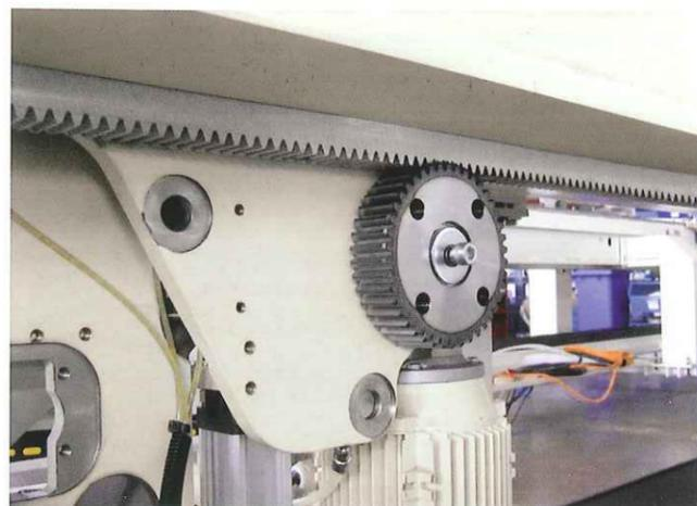
**SAW CARRIAGE MOVEMENT BY RACK AND PINION SYSTEM**
