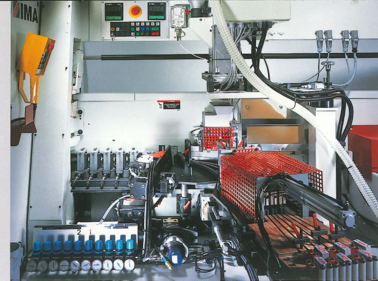
Abb.: Verleimaggreat 283.1513 – Novimat CONCEPT [Verleimaggreat 04.1570 – Novimat CONCEPT – R]
