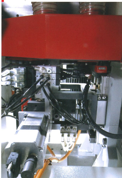
Joint milling unit 08.378
