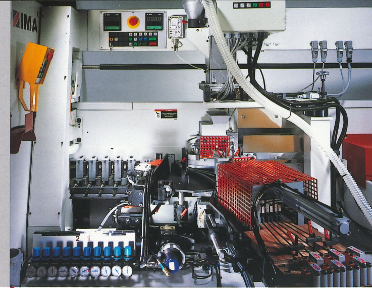
Novimat CONCEPT – edge banding unit 283.1513 (picture) [Novimat CONCEPT – R – edge banding unit 04.1570]
