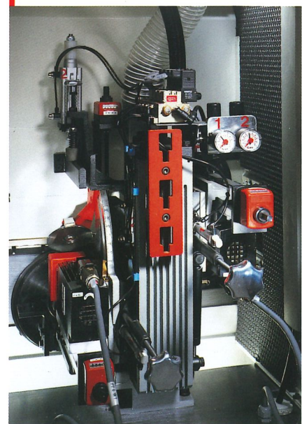
Fine-/Profile milling unit 08.055
