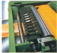
Stock Control With Safety Sectional chip breaker over the whole width of material. And anti kickback fingers fitted as standard.
