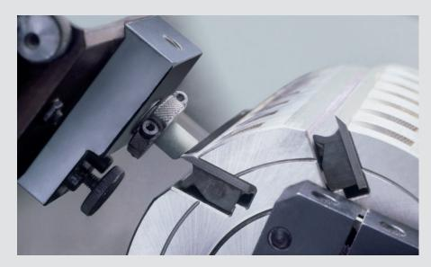
Remotely controlled fully automatic profile jointer with automatic joint stone infeed.
