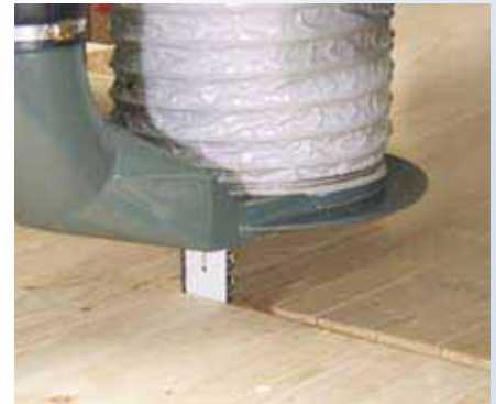
Sawing with up to approx. 350mm depth
