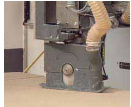
Sawing at max. approx. 30m/min
