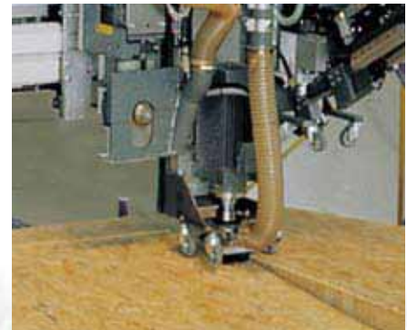
Milling at up to approx. 25m/min
