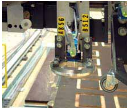
Marking/labelling with inkjet/colour pen or scriber
