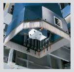
Multi-spindle routing unit In L-shape, 9 spindles, individually selectable
