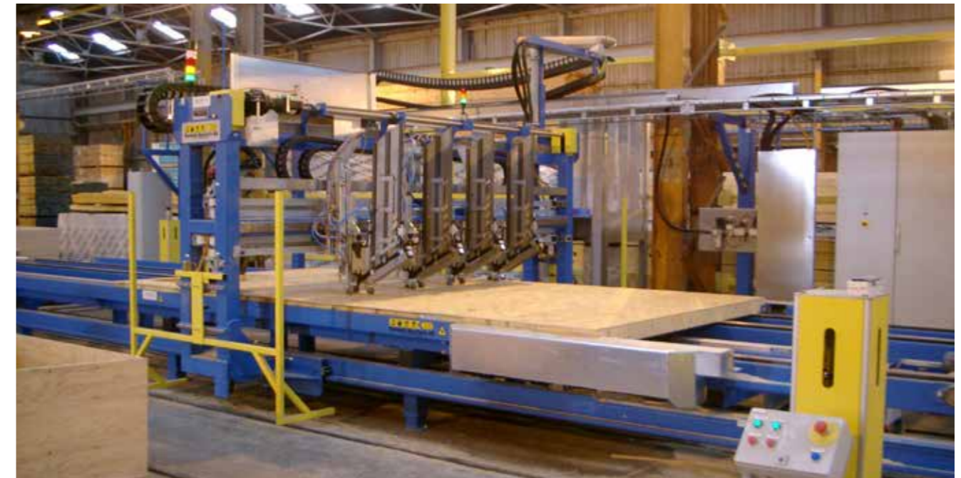
A CAD/CAM-controlled nailing bridge can be used or a manual NB1000F
