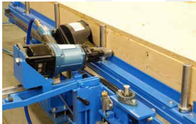
The framing table is equipped with weight balanced nailing wagons running along the station for safe and exact nailing of the timber frame work.
