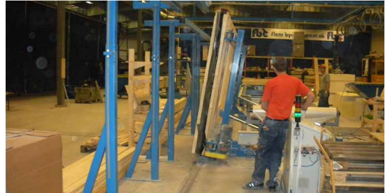
The wall element is erected and fed to Vertical Outfeed System directly from Combi System for effective mounting of windows etc.
