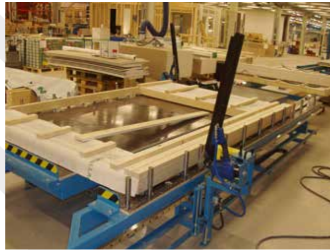
Weight balanced nailing wagon on a Framing Table FT2000
