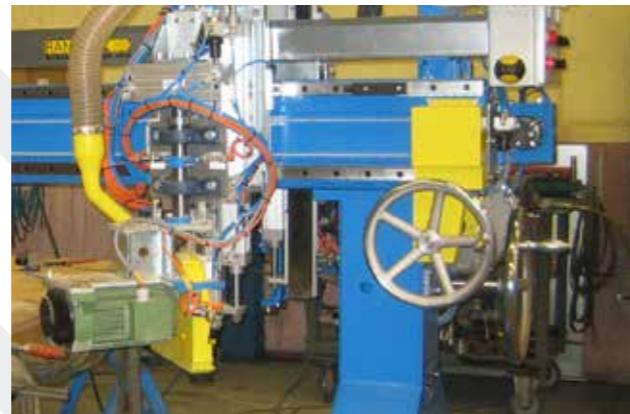
It is possible to install a manual Nailing bridge NB1000, seen above, or a CAD/CAM-controlled Nailing bridge NB3000.
