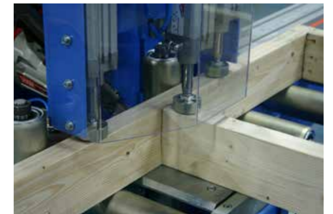
Close view of the clamping system on FM1000TS the system enables timber frame production with high quality and capacity.
