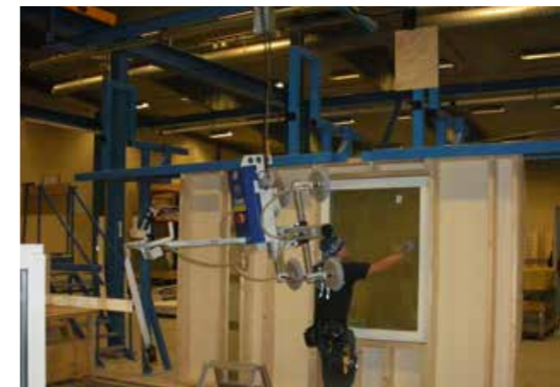
Effective window mounting in a Vertical Outfeed System.
