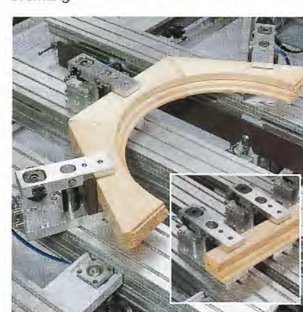
A lot of clamping systems are available for narrow or frame parts.
