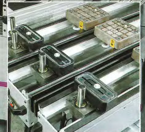
Standard: 2 nd row of stops (front) as well as 8 narrow vacuum cups.
