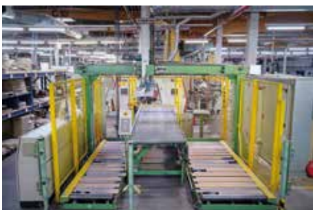
SYSTRAPLAN Feeding and destacking unit Year of construction 1994
