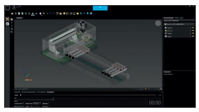
B\_SOLID makes the customer's machine available in a virtual environment, complete with its components and the NC axis movement kinematics.
