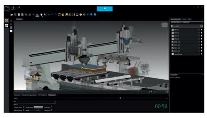
Simulation is not only handy when it comes to checking or preventing collisions; it also enables a calculation of the time needed to carry out all the machining operations, thereby facilitating the factory logistics system.
