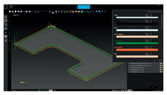
Automatic generation of the edgebanding operation sequence (pre-edgebanding, edgebanding, post-edgebanding).
