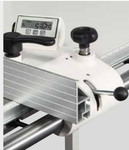
Reversible rip fence, available on request, with heavy duty cast iron support sliding over a rectified steel round bar, equipped with rack & pinion micrometric adjustment and cam-lock system.
