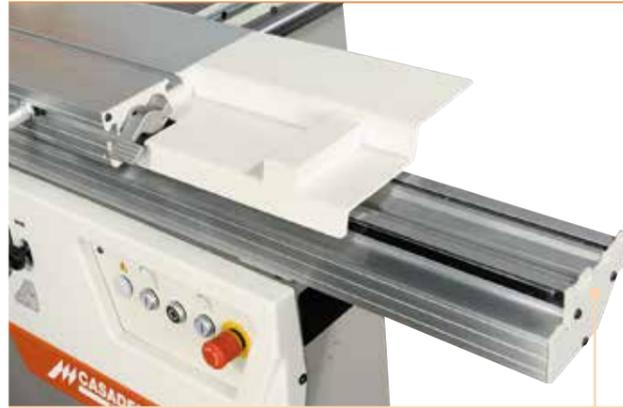
Hardened steel guideways with double prismatic guideway and preloaded ball bearings. Precision, smooth running and absence of maintenance are unique features of the CASADEI sliding table.
