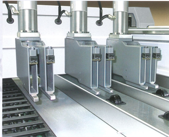
Spezial-Spannzangen – vertikale Spannkraft für alle Pakethöhen. Heavy duty clamps – vertical clamping motion with uniform pressure for every book height.
