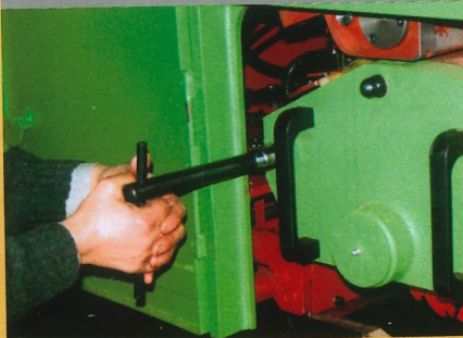
Disassembly the side door with outboard bearing
