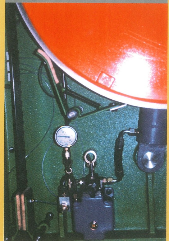
Detail of the hydraulic blade tension
