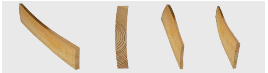
Blocks with longitudinal/latitudinal deformation, cupped or warped
