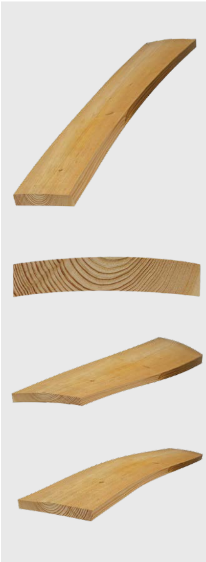
Blocks with longitudinal/latitudinal deformation, cupped or warped
