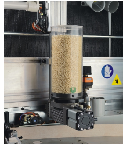
Pre-melting system QM-705 for EVA glue. EVA 胶水快速预溶装置 QM-705
