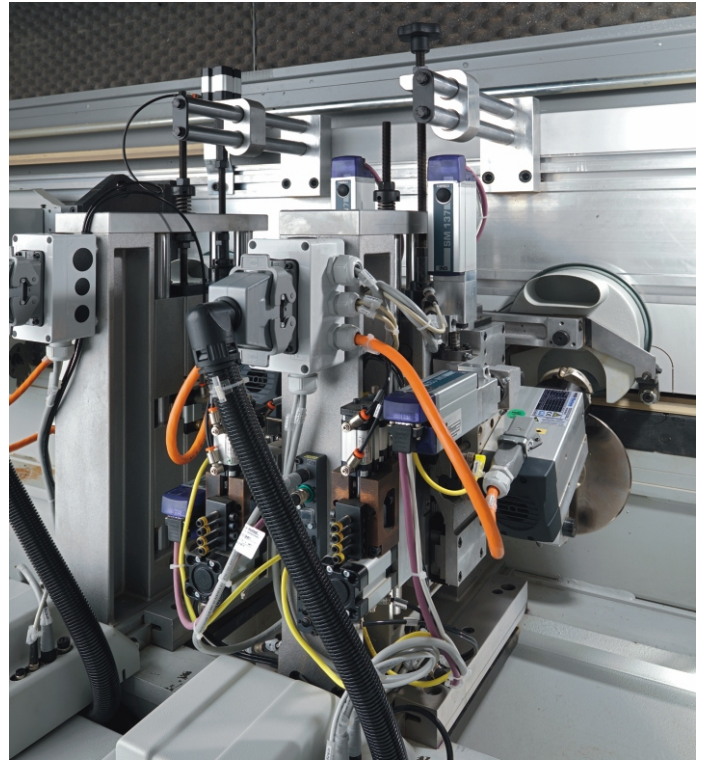
Multifunction Tilting top and bottom chamfering unit RF-400.
