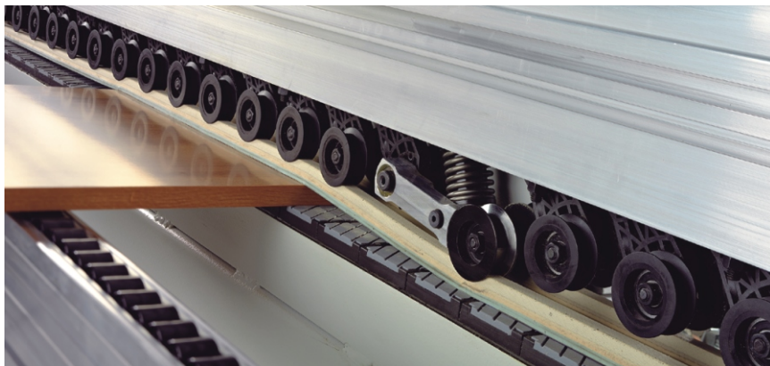
Belt presser for an optimal cleaning of the panel. (Opt.)
