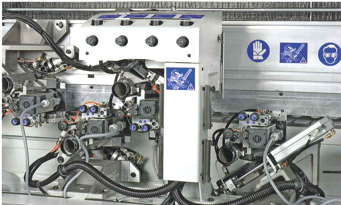
Multifunction 4 motors Rounder CR-401 (standard 4 positions FAST system).
