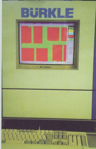
PC für Multi-Pin System zeigt Legebild an PC for the Multi-Pin System to show the lay-up pattern
