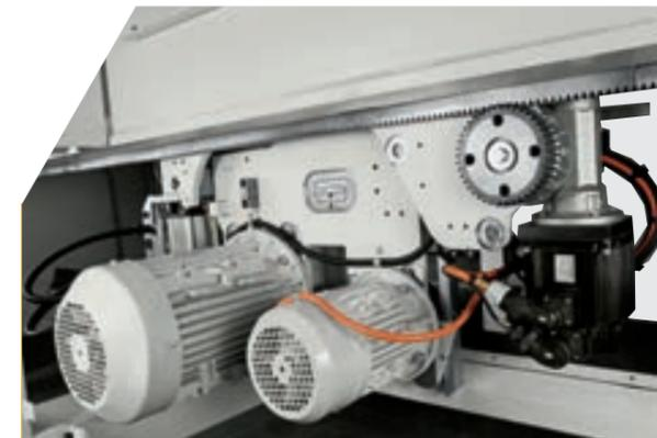
Rack & pinion saw carriage feed system: speed and accuracy.
