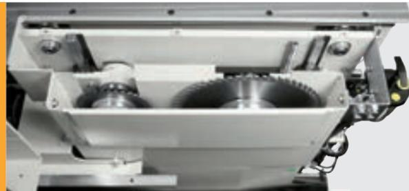
Standard saw carriage with 2 linear, prismatic guides
