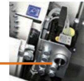
Pneumatic flanges locking/unlocking for
