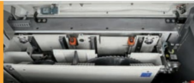
Optional saw carriage with 4 linear, prismatic guide (standard for HD version)
