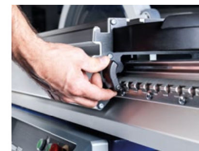
Fix in every position – Multiple position locking of the sliding table
