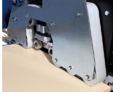
Continuous transport of the workpiece
