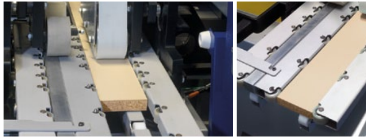
Workpiece widths between 70–920 mm
