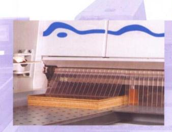
To minimise each cutting cycle, an electronic control limits the movement of the steel pressure beam and a flap type safety curtain is used that remains on the panel during the cutting sequence, thus eliminating wasted travelling time.
