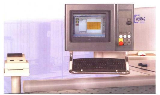
A modern PC controls all the movements of the saw and functions using a comfortable user interface between man and machine with graphical support for all functions offering quick access to the whole range of operations available on a modern panel saw.
