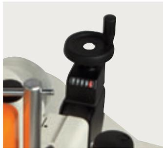
The entire fence and its feed fence are set up and adjusted with respect to the tool, thanks to the handwheels and the relevant mechanical digital readouts.
