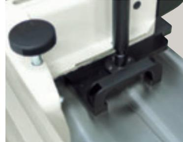
The fence repositioning on the table in the previous position is rapid and precise thanks to the two reference pins.
