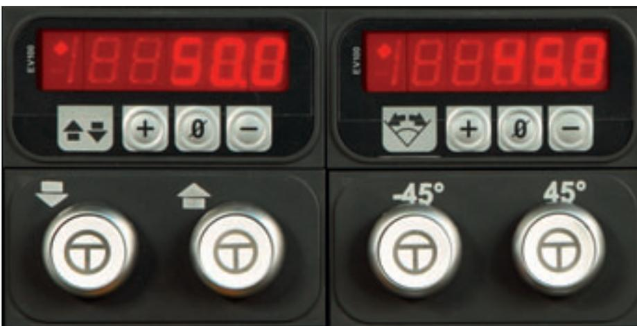
Electromechanical pushbuttons from control panel on machine front are used to adjust the spindle setting in relation to the worktable. The electronic digital readouts ensure accurate set-up to one-tenth of a millimetre precision. Precision set-up means that trial runs are reduced to the minimum.
