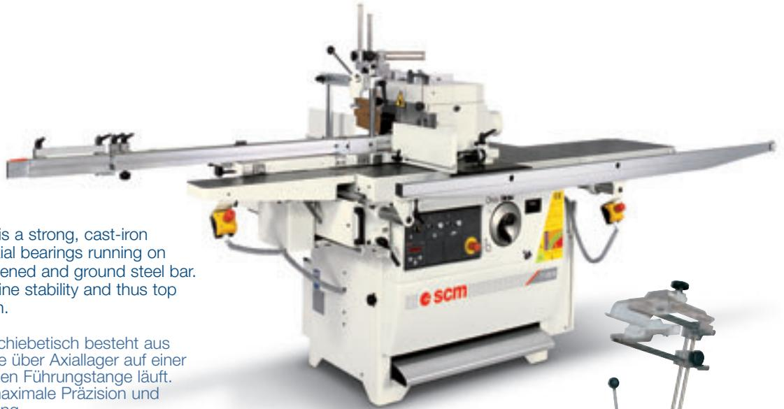
The manual feed carriage is a strong, cast-iron framework mounted on axial bearings running on slideways made from hardened and ground steel bar. This guarantees top machine stability and thus top quality machining precision.
