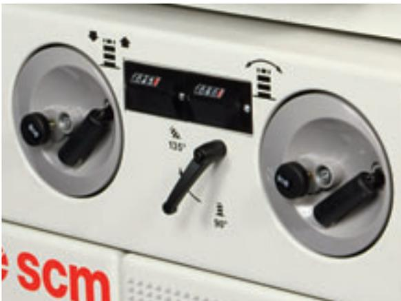
A handwheel positioned on machine front is used to adjust the spindle setting in relation to the worktable. The mechanical numeric indicators ensure accurate set-up to one-tenth of a millimetre precision. Precision set-up means that trial runs are reduced to the minimum.
