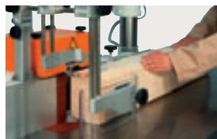
It grants higher operator's safety as the processed workpiece is positioned between the rotating tool and the operator.
