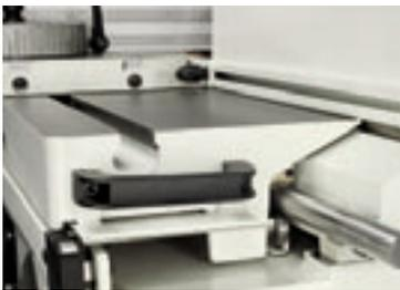
The hardened steel bar, on which the tenoning carriage runs (by means of bearings), grants a perfect machinings repeatability and movement linearity.
