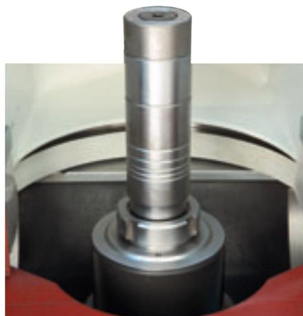
**Interchangeable spindle with MK5 tool taper** to use a tool for a different worktable hole diameter, just change the tool spindle.
