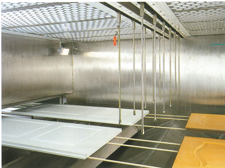
Inner view of spray cabin with coolac® paint recovery system for water-based paints
