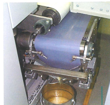
The new 'V-belt lacquer recovery system'
