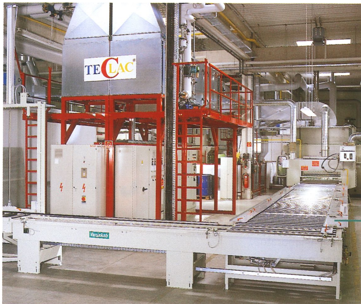
Surface installation for coating of plastic car parts
