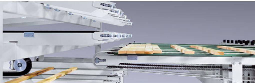
The powerful accelerator keeps the scanner supplied with material. Speeds of over 270 m/min guarantee reliable loading of the cross-cut saws. The solid design minimises vibration during transport, thus ensuring a high standard of detection by the scanner. Sophisticated mechanisation and automatic stacking guarantee high productivity.
