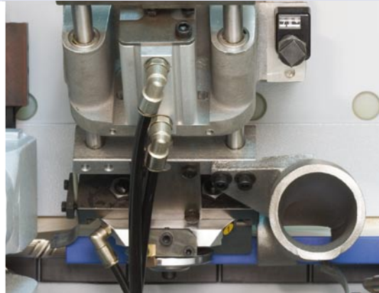
Pneumatic horizontal displacement for PN 10/FA 11
