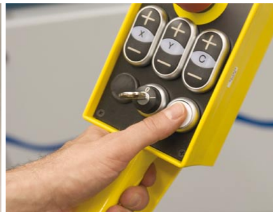
A remote control facility for single-sided machines permits fast set-up
