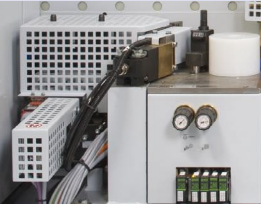
Automatic program-based adjustment of the pressure zone in line with the relevant edging thickness
