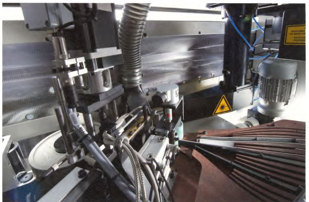
The heart of the Laser Edging process: a highly accurate laser beam and the pressure roller station
